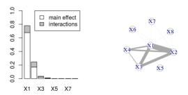
Figure: 1st order analysis (left) and 2nd order analysis (right) with 10<sup>5</sup> simulated data
